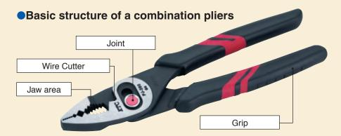
The head is of a curved shape, and a wave-shaped tooth inside to prevent materials from slipping. The tip of the jaw area is flat, and the center is curved to ease the gripping of poles and pipes. The mouth size can be adjusted by shifting the joint area (fulcrum).
