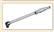
The square drive can bend left or right up to 90° about a pin in the center of the head part of the shank and stop at a given angle. When turning quickly to temporarily tighten and so on, the handle can be held straight and used like a screw driver (Fig. 1), and when tightening securely, a strong torque can be generated by holding the handle to the side (Fig. 2).
