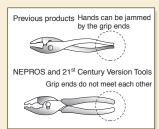
The combination pliers is a convenient tool for various purposes. However, it is important to use the correct tools for specific operations. Using the combination pliers for the tightening/loosening of nuts and bolts and the cutting of large, hard wires may cause damage. Use the offset wrench or socket wrench for tightening/loosening nuts and bolts, and the nippers or wire cutters for cutting hard wires. It is important to use the correct tool to suit each of the operations detailed here.
