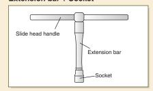
The slide head handle can be used as a "T shaped handle" in combination with an extension bar. By adding a ratchet adapter between the slide head handle and the extension bar, it can be used as a "T shaped ratchet".
